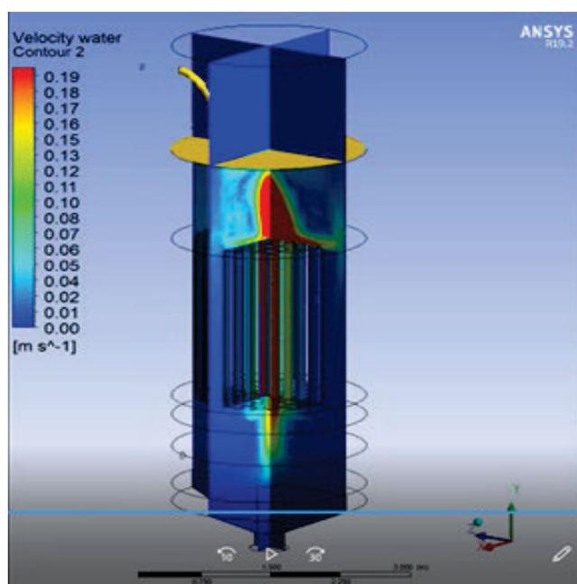
**Fig. 3.** Numerical evaluation of the flow in the bioreactor – the dominant flow in the bed core and the autocyclic flow in the opposite direction in the peripheral areas of the adhesive bed; source: own study
