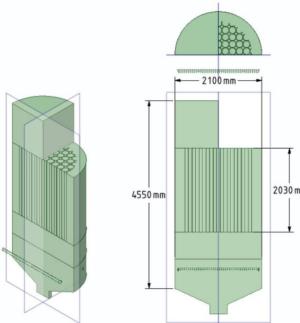
**Fig. 1.** Geometry of the analysed fermenter: upper part – storage area of the produced biogas; middle part – adhesive bed forms a skeleton composed of 72 pipes; lower part – fermenter drain; source: own elaboration
