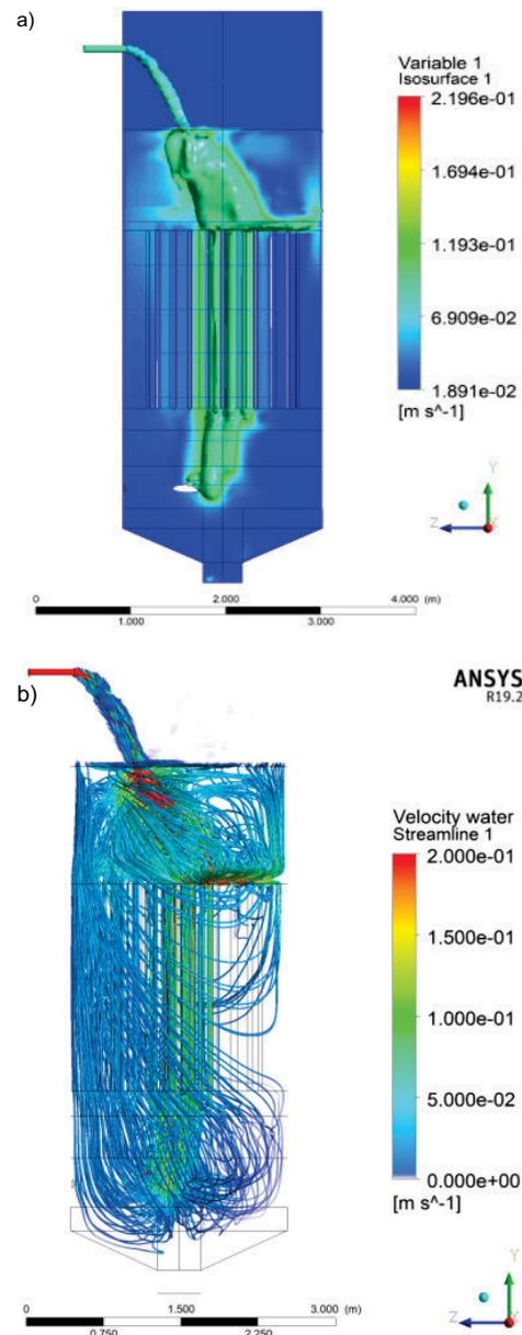
**Fig. 2.** Numerical evaluation of the flow in the bioreactor: a) velocity iso-surface: qualitative representation of the main mixing range and the location where the highest speeds occur; b) streamlines – view of the recirculation zone; source: own study
