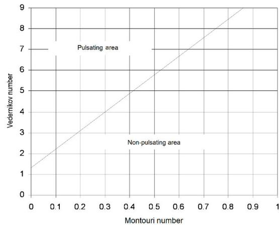
Fig. 3. Pulsating flow criteria graph; source: USBR [1987]
