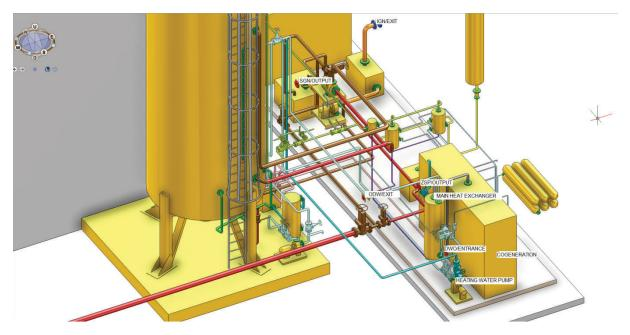
**Fig. 5**. Visualisation – AVEVA 3D Integrator – fragment of the biogas production installation, integration of the diagram with the model environment and creation of pipelines using Integrator mechanisms; red = substrate flow, IGN/EXIT = digestate outlet, SGN/OUTPUT = digestate inlet, ZSP/OUTPUT = hot water outlet, ODW/EXIT = substrate outlet, DWO/ENTRANCE = water inlet to be heated; source: own study based on AVEVA (2020)
