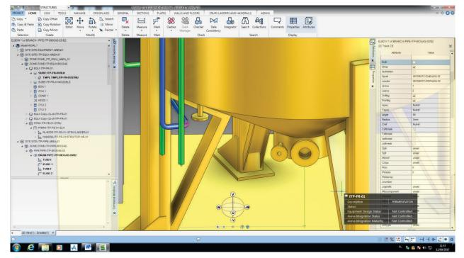
Fig. 3. Visualisation – AVEVA 3D Integrator – fragment of the bottom of the fermenter, P&ID diagram and 3D model; source: own study using AVEVA (2020)
