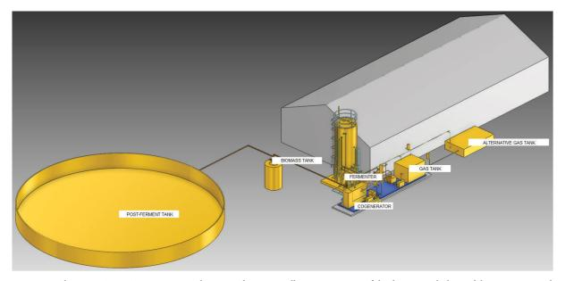
Fig. 4. Visualisation – AVEVA 3D Integrator – biogas production installation, integration of the diagram with the model environment and creation of pipelines using Integrator mechanisms; source: own study based on AVEVA (2020)
