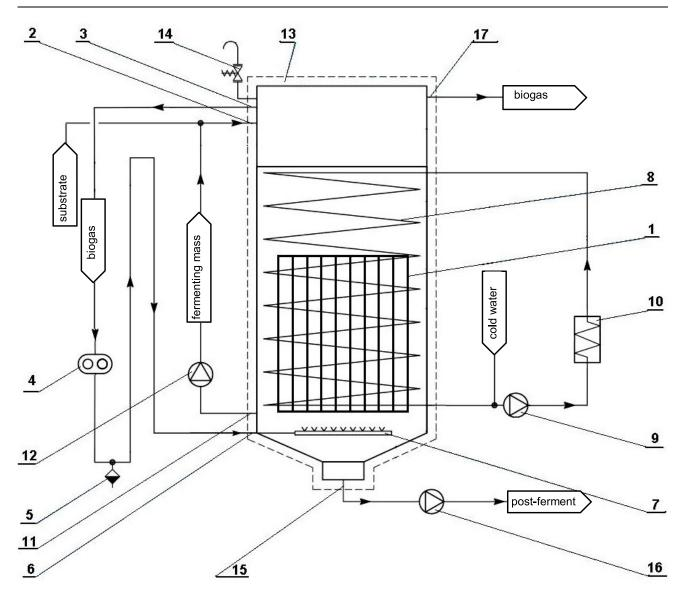
**Fig. 2.** Diagram of the fermenter: 1 = pipe, 2 = connector, 3 = biogas outlet connector, 4 = blower, 5 = biogas drainage valve, 6 = biogas outlet connector, 7 = bubbler, 8 = heating coil, 9 = water pump, 10 = heat exchanger, 11 = fermenting mass outlet port, 12 = fermenting mass pump, 13 = thermal insulation, 14 = safety valve, 15 = main digestate outlet port, 16 = digestate pump, 17 = biogas outlet port; source: Myczko *et al.*, 2018.
