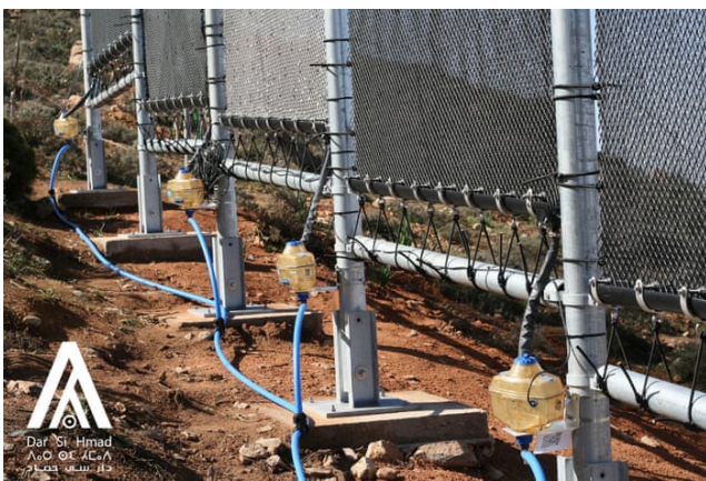
Photo 4. Nets capture moisture which is collected and filtered then mixed with underground water (phot.: Dar Si Hmad)
