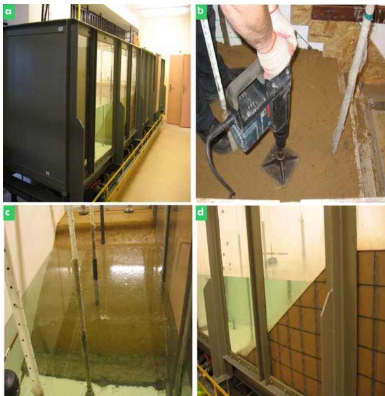
Photo 1. Medium-size apparatus for testing filtration through embankment models; a) front wall view, b) soil compaction in the model, c), d) damming water by the model (phot. M. Cholewa )
