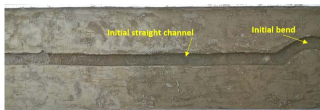
Fig. 2. Initial straight channel with an initial bend prepared for experiment; source: own elaboration
