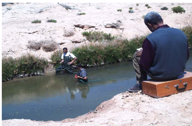
Photo 3. Flow velocity measurements near the left bank of the channel (phot. M. Sayah Lembarek)
