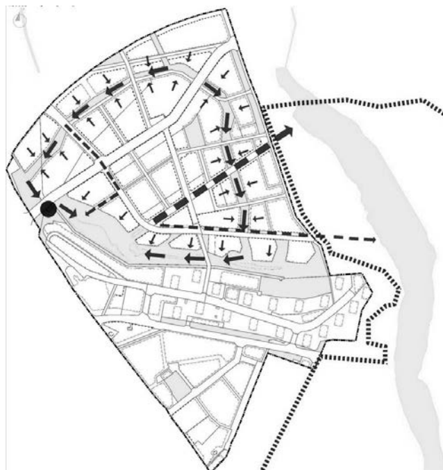
Fig. 2. A diagram of the planned rainwater collection system in Czerniaków Południowy area and supplying Lake Czerniakowskie with water – a “green horseshoe”; the arrows indicate the direction of water flow; source: own study
