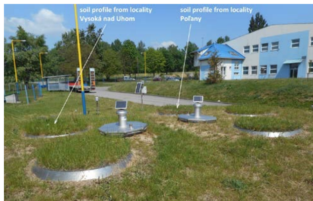
Fig. 1. Lysimeter station in Petrovce nad Laborcom; source: own elaboration, phot. A. Tall
